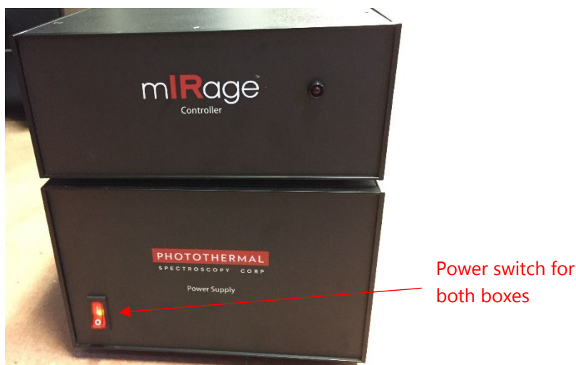
Figure 2-5. The mIRage controller and power supply.
