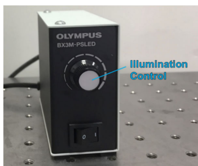
Figure 2-9. The Olympus power supply
