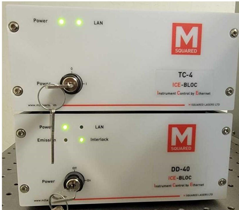
Figure 2-11 OPO IR laser controller boxes
